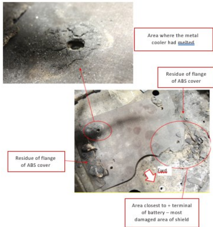
Figure 11: phenolic shield on aeroplane floor (source: BEA)
