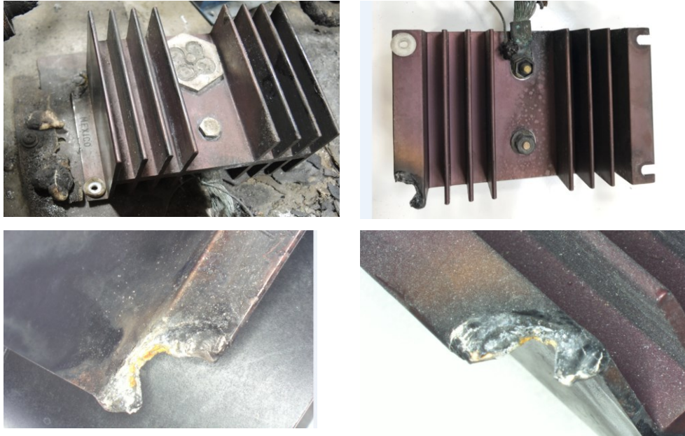
Figure 10: metal cooler of diode device after disassembly (source: BEA)
