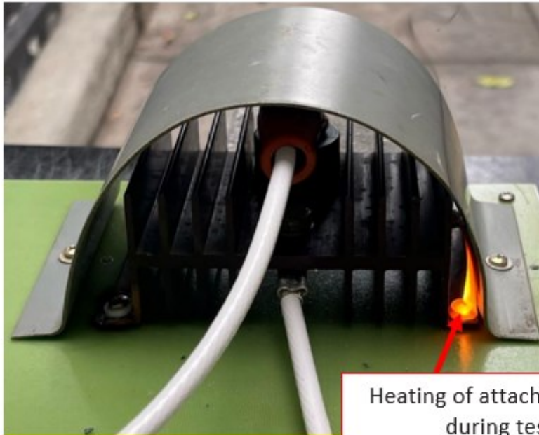
Figure 18: ABS cover in position with attaching point subject to intense heat (source: CONCORDE BATTERY CORPORATION)
