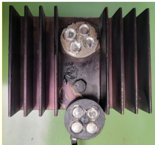
Figure 21: separation of diode bridge from metal cooler (Source: CONCORDE BATTERY CORPORATION)
