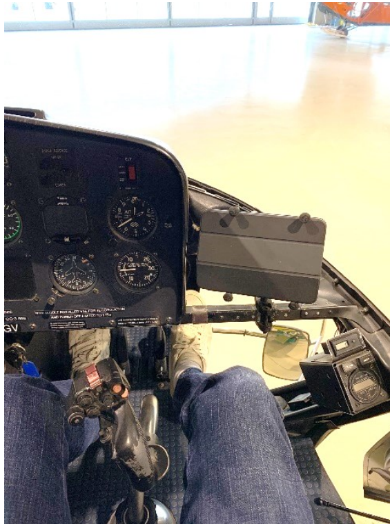
Figure 5: mount used by Eagle Valais and removed by the pilot (source: BEA)
