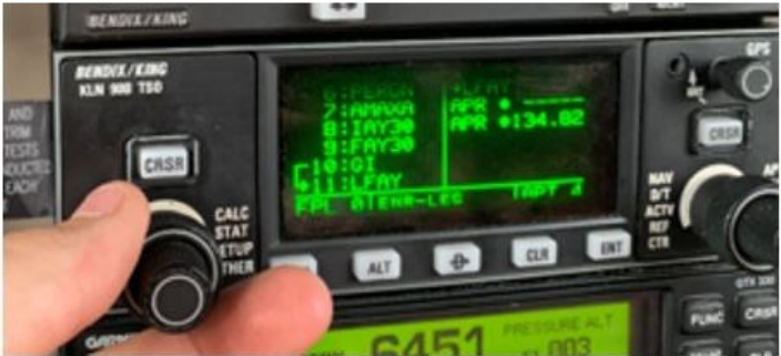
GNSS Bendix KING 90 (page of RNP30 approach waypoints)
