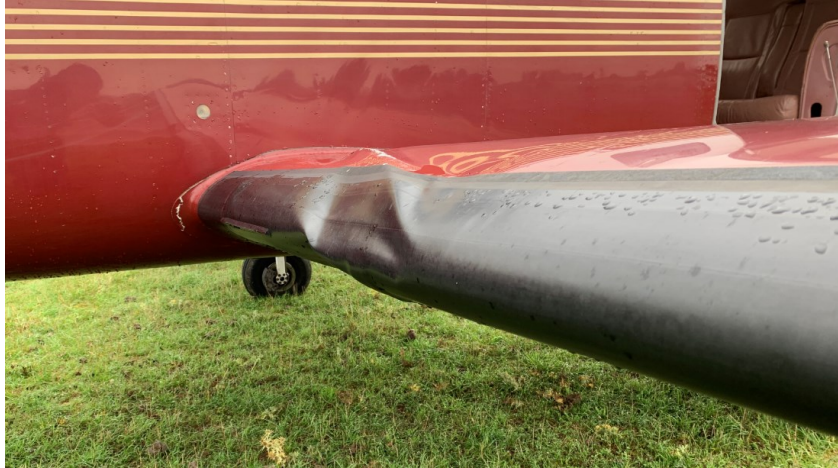
Figure 3: damage to wing roots of N9190X (Source: BEA)
