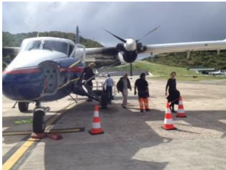
Figure 3: position of cones around engines (source: safety booklet)
