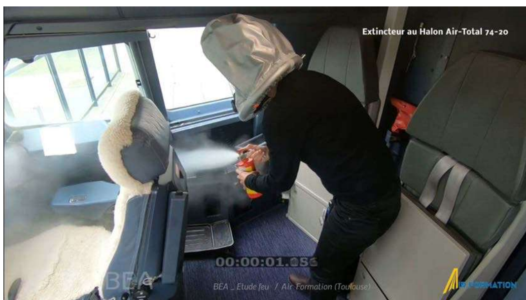
Activation of a cockpit fire extinguisher in the cockpit of Air Formation's A340
