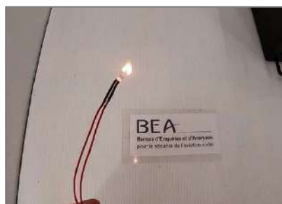
Figure 35: spark production device (source: BEA)
