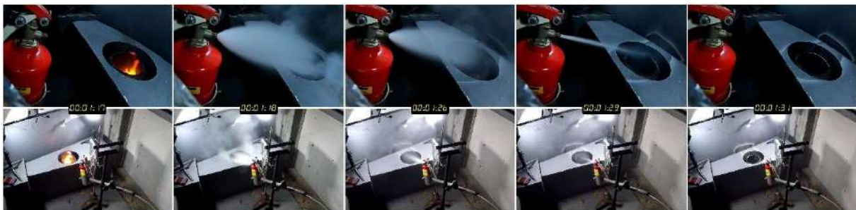
Figure 49: extinguisher_01 test - video sequence (source: BEA)
