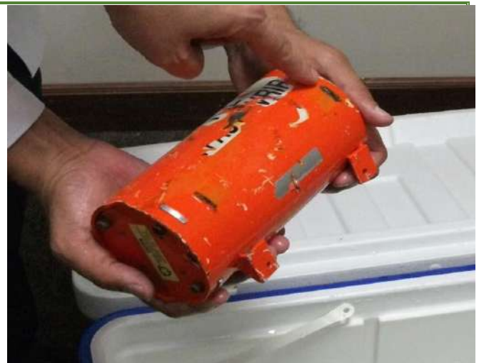
Figure 1.11/5: Two of four mounting brackets missing
