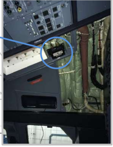
Pre-amplifier (CU hidden under a cover panel).
