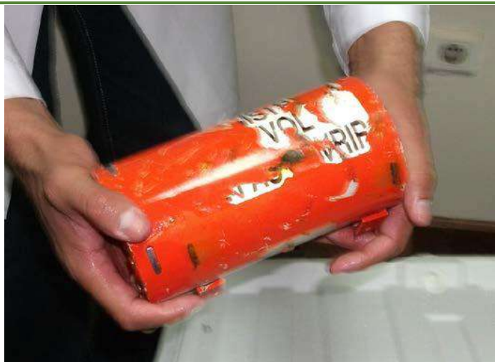
Figure 1.11/4 : Missing decals, paint chips and gouges in the CSMU
