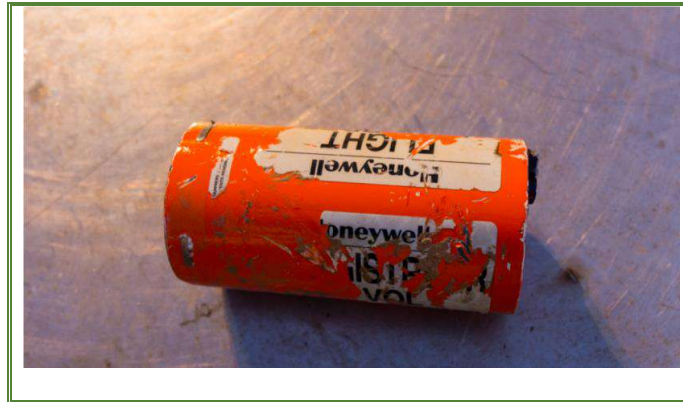
Figure 1.12/6: The CSMU memory unit belonging to one of the aircraft recorders after being recovered
