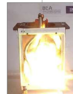
Oxygen box assembly catches fire
