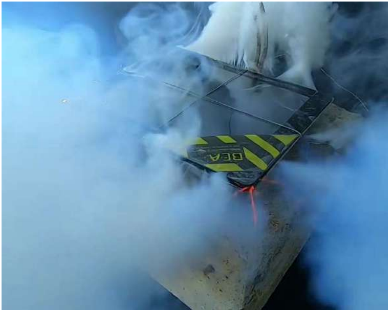
Figure 24: example of release of smoke during thermal runaway of battery (Lithium_Battery_04 test)
