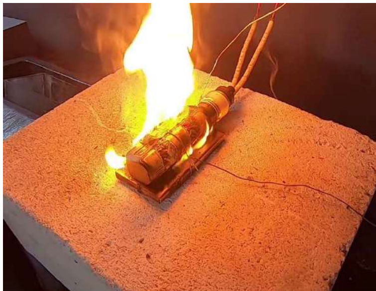
Figure 26: visible flames during Lithium_Battery_07 test
