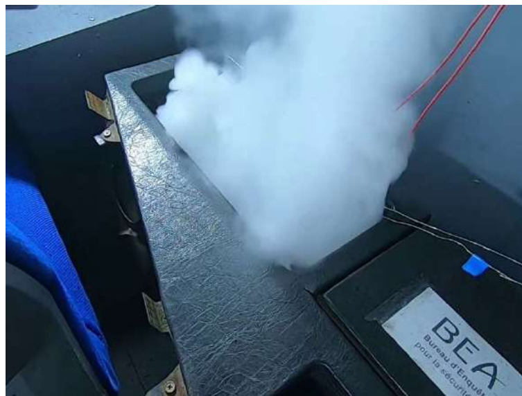
Figure 27: release of smoke during Lithium_Battery_05 test
