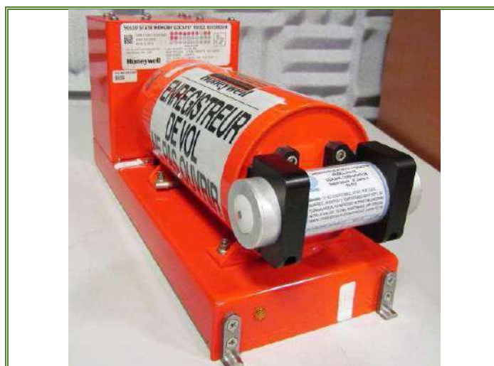
Figure 1.11/8: Example of undamaged Honeywell 980-6022-XXX recorder
