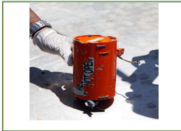
Figure 1.12/4: The CSMU memory unit belonging to one of flight recorders after being recovered.
