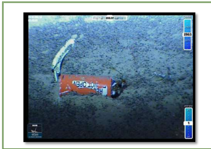
Figure 1.12/3: The memory unit belonging to one of the aircraft flight recorders at the depth of 3020 meter from the sea surface
