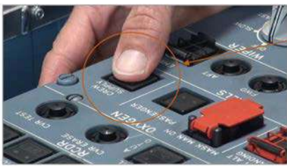
Electrical control of oxygen supply valve
