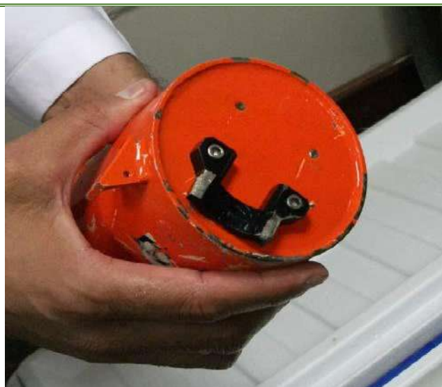
Figure 1.11/7:ULB bracket failure and the second bracket missing
