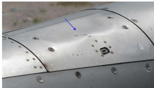
Figure 19 - Dent on the overpressure panel
