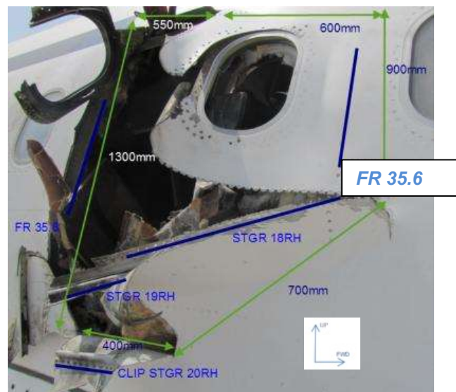
Figure 7 - Skin damaged dimension
