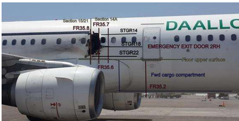
General view of the fuselage perforated area
