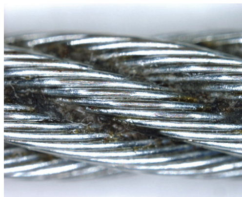
Binocular view of the wear area on a carbon steel cable after 150,000 cycles
