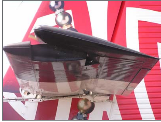
Elevator in locked position
