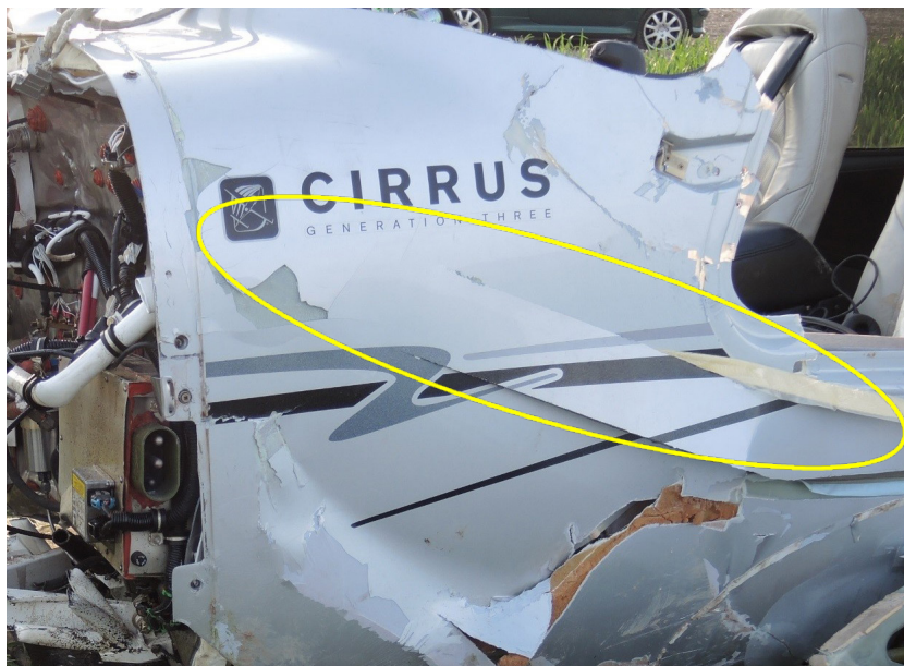
Figure 1: lateral strap of emergency parachute on left side
