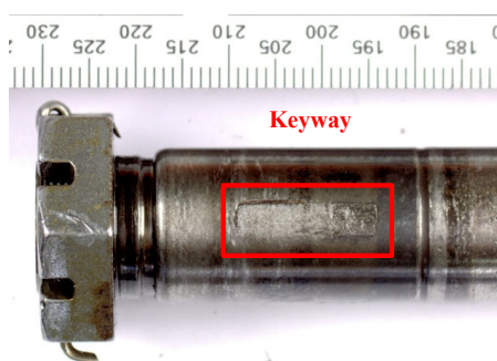
Figure 8: Keyway on alternator shaft side
