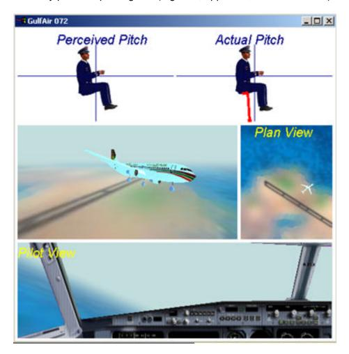
**Figure 1**: Perceived Pitch versus Actual Pitch just prior to stick forward (t=1929:43) (Red Arrows in Actual Pitch panel are the Gx and Gz acceleration vectors)
