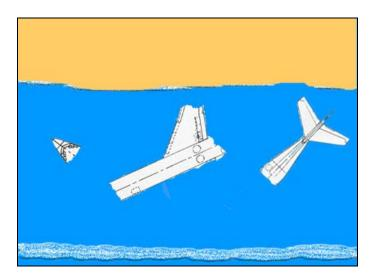
The main part of the airplane had turned over and only the lower part of the fuselage and the underside of the left wing were visible. Both of the outer engines had separated from the tail.
