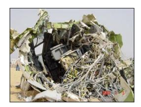
The cockpit was not very damaged, except for the Flight engineer's panel and a large part of the equipment. There was a strong compression mark on the floor and the skin of the partition and the outer right side of the fuselage. The nose gear had been ripped off.
