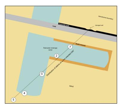
The plan of site 2 shows the position of the parts found in the rain drainage channel that crossed it. The heavy parts, numbered ① to ⑤ indicate the airplane's path after it passed over the aerodrome boundary wall.
