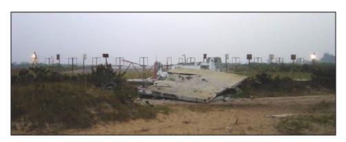
Damage on the right was noted that was caused by the right main landing gear, on the central part marks were left by the lower part of the fuselage and on the left side there was damage caused by the left main landing gear.
