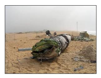
The majority of engine 3 was intact. The thrust reverser was still attached to the engine, in the retracted position. No damage due to a fire or an uncontained burst was noted.
