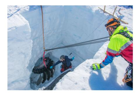
Extraction of part of the fan hub found 4 m under the surface of the Greenland ice sheet in June 2019 - Photo by Austin Lines
