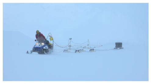
Testing the operation of the electromagnetic system, SnowTEM, on a glacier at Zermatt (Switzerland) in January 2019
