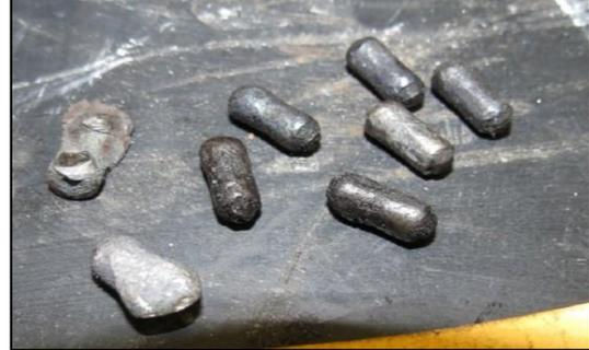
Figure 2-7 : No 6 Bearing Rollers
