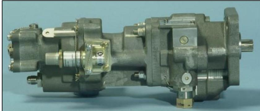
Figure 1-103: OSG and the Main Pump
