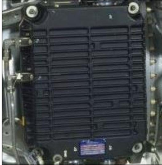
Figure 1-93: Electronic Engine Control
